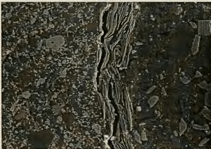
Figure 4.27 Scanning Electron Image of metallic layer in sample 1.04-6 from the living room metallic finish. The center line is the location of the metallic finish in the sample.
